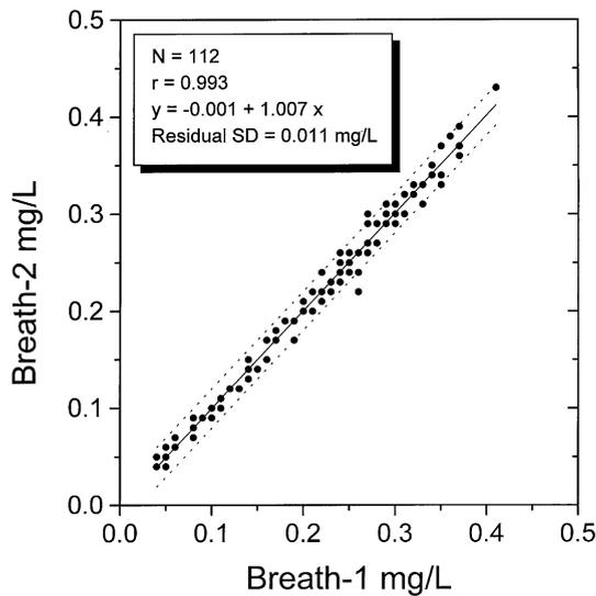
Fig. 2. Association between duplicate breath-alcohol measurements, where  $N$  is number of  $x$ - $y$  pairs,  $r$  is the correlation coefficient and S.D. is residual standard deviation or random error. The regression equation was  $\text{BrAC-2} = -0.001 + 1.007 \text{ BrAC-1}$ .
